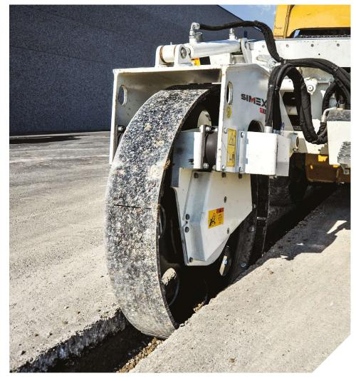
Counter-rotating vibrating double shaft
